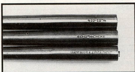
Barrel markings of the .410 bore H&R Handy-Gun: Model 1, Types I, II and III, and Model 2, Type I are 410-12m/m (top); for Model 2, Type II are 410-12m/m CHOKE (middle); and for Model 2, Type III, and Model 3, Types I, II and III are MADE IN U.S.A. 410 GA. CHOKE (bottom).
